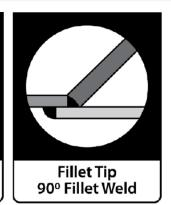
Fillet tips are used mainly for fillet welds [90°] and butt welds. The style of those tips allows one to weld from inside corners out and be able to seal the corners without changing to another tip style. Fillet tips can also be used for crack repairs, as long as the crack is somewhat straight. The longer preheat section allows faster welding speed than welding cracks with the conical tip.
